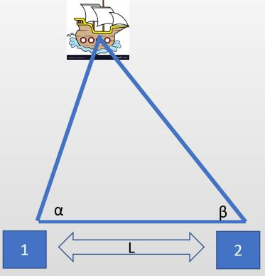
Two observers can "triangulate" the location of the boat (distance from the short) by measuring the angles  $\alpha$  and  $\beta$ , using the distance L and the law of sines.
